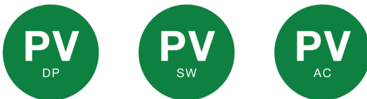
Figure 9. Example of fire and emergency information signs: See Appendix A3 in AS/NZS 5033:2021
