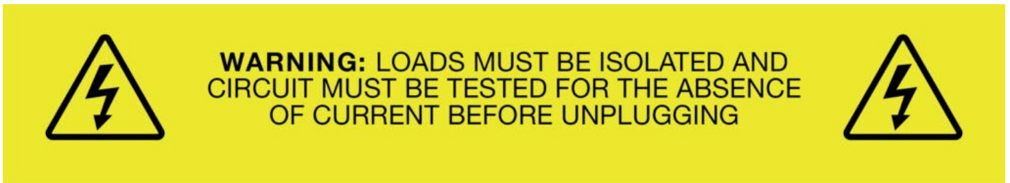
Figure 10. Disconnection point sign: See Appendix A4(c) in AS/NZS 5033:2021
